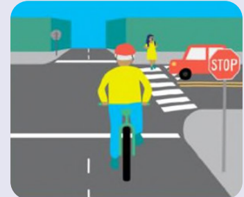
LTS 3: Marked crosswalk on one side without crossing signal
