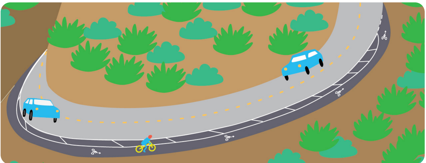
Separate space for a bicycle as a "bike turnout" for uphill, bend section of a road.
