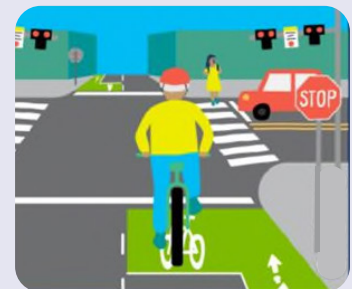
LTS 1: Marked crossing with specific accommodations for both walking and bicycling
